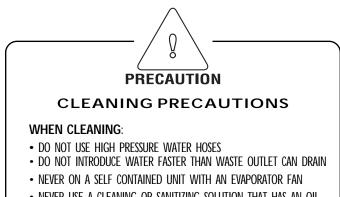
• NEVER USE A CLEANING OR SANITIZING SOLUTION THAT HAS AN OIL BASE (these will dissolve the butyl sealants) or an AMMONIA BASE (this will corrode the copper components of the case)
